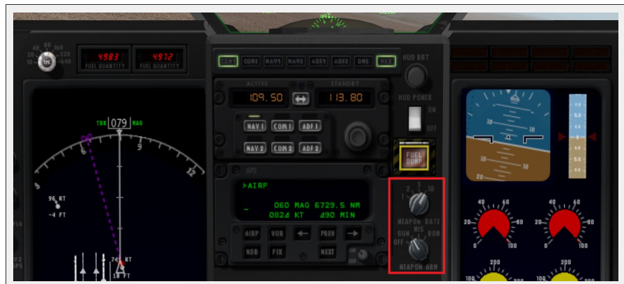
Figure 8.5: The weapon controls in the panel of the F-22 Raptor [Full size →]
