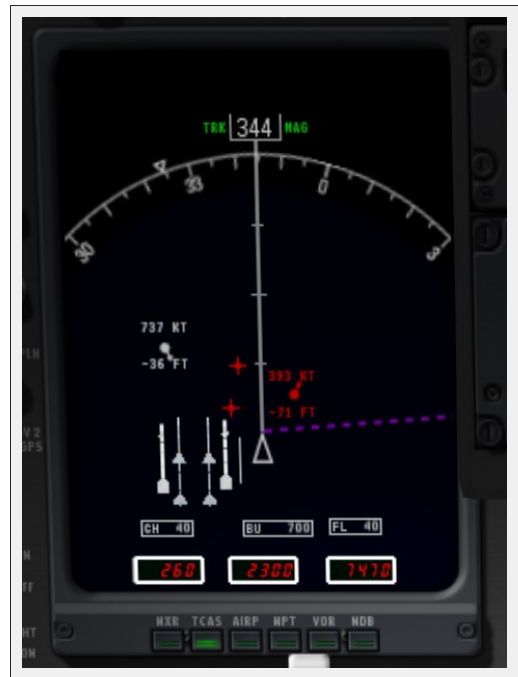
Figure 8.9: The moving map display with a target selected, located about 30 degrees to the right, in front of the aircraft and travelling at 393 kts [Full size →]
