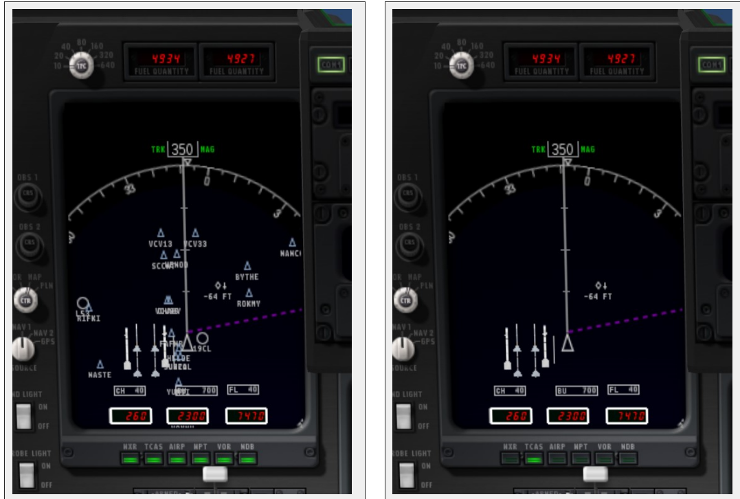
Figure 8.8: Two moving map displays; the display on the left is showing all available data, whereas the one on the right is showing only other aircraft [Full size 1 →] [Full size 2 →]
