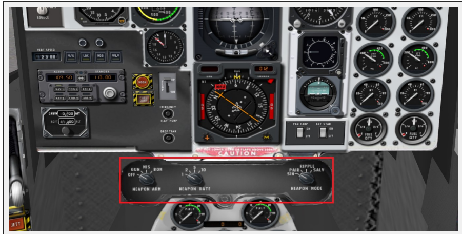
Figure 8.6: The weapon controls in the panel of the F-4 Phantom II [Full size →]
